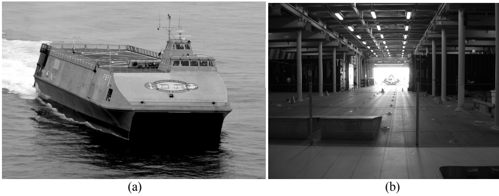
Figure 1. The high-speed aluminum littoral combat ship FSF-1 SeaFighter: (a) SeaFighter at sea; (b) the internal mission bay featuring open spaces on the ship main deck.
